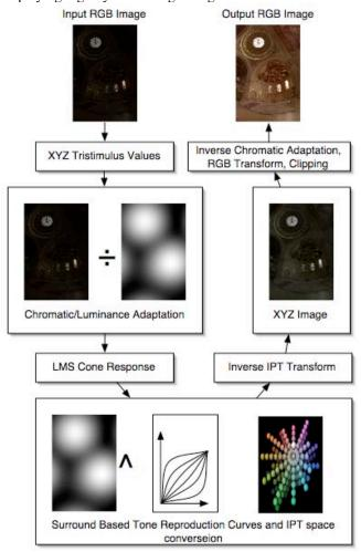
Figure 1. Flow chart of iCAM for rendering high dynamic range images.
