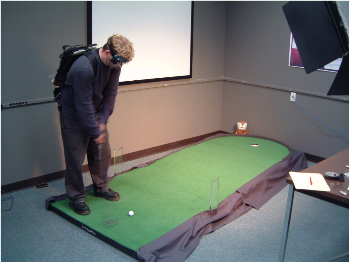
Figure 1. The putting green configuration in use during these experiments. Note the diffuse bluish simulated daylight illumination and the direct yellowish simulated sunlight illumination. This golfer is wearing the portable eye-tracking system.
